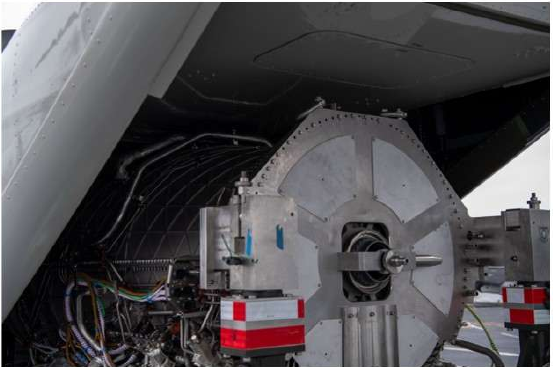
210211-N-MD461-1181 PACIFIC OCEAN (Feb. 11, 2021) An F-35C Lightning II power module is loaded onto a CMV-22B Osprey assigned to the "Titans" of Fleet Logistics Multi-Mission Squadron (VRM) 30 on the flight deck of Nimitz-class nuclear aircraft carrier USS Carl Vinson (CVN 70). Vinson is currently underway conducting routine maritime operations. (U.S. Navy photo by Mass Communication Specialist Seaman Jeffrey Kempton/Released)
