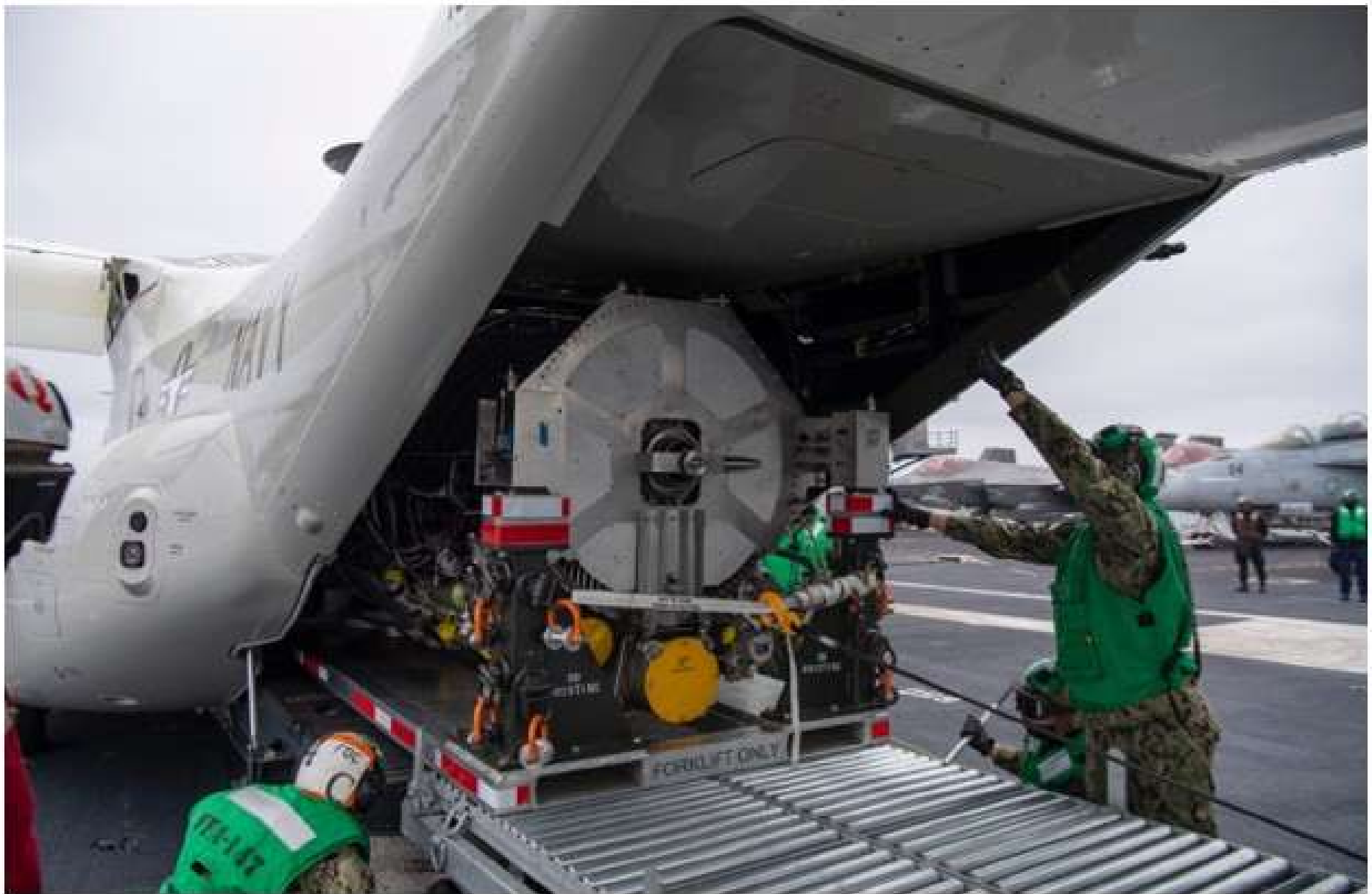
210211-N-MD461-1202 PACIFIC OCEAN (Feb. 11, 2021) Sailors assigned to the “Argonauts” of Strike Fighter Squadron (VFA) 147 load an F-35C Lightning II power module onto a CMV-22B Osprey assigned to the “Titans” of Fleet Logistics Multi-Mission Squadron (VRM) 30 on the flight deck of Nimitz-class nuclear aircraft carrier USS Carl Vinson (CVN 70). Vinson is currently underway conducting routine maritime operations. (U.S. Navy photo by Mass Communication Specialist Seaman Jeffrey Kempton/Released)
