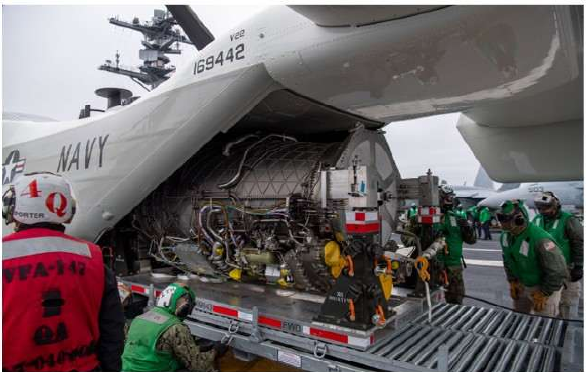
210211-N-MD461-1165 PACIFIC OCEAN (Feb. 11, 2021) Sailors assigned to the “Argonauts” of Strike Fighter Squadron (VFA) 147 load an F-35C Lightning II power module onto a CMV-22B Osprey assigned to the “Titans” of Fleet Logistics Multi-Mission Squadron (VRM) 30 on the flight deck of Nimitz-class nuclear aircraft carrier USS Carl Vinson (CVN 70). Vinson is currently underway conducting routine maritime operations. (U.S. Navy photo by Mass Communication Specialist Seaman Jeffrey Kempton/Released)
