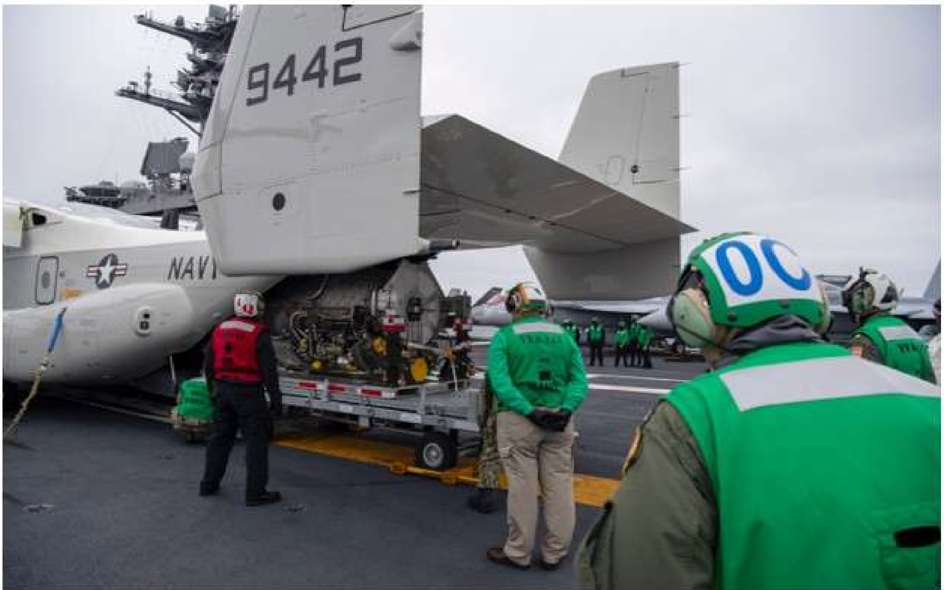
210211-N-MD461-1155 PACIFIC OCEAN (Feb. 11, 2021) Sailors assigned to the “Argonauts” of Strike Fighter Squadron (VFA) 147 load an F-35C Lightning II power module onto a CMV-22B Osprey assigned to the “Titans” of Fleet Logistics Multi-Mission Squadron (VRM) 30 on the flight deck of Nimitz-class nuclear aircraft carrier USS Carl Vinson (CVN 70). Vinson is currently underway conducting routine maritime operations. (U.S. Navy photo by Mass Communication Specialist Seaman Jeffrey Kempton/Released)
