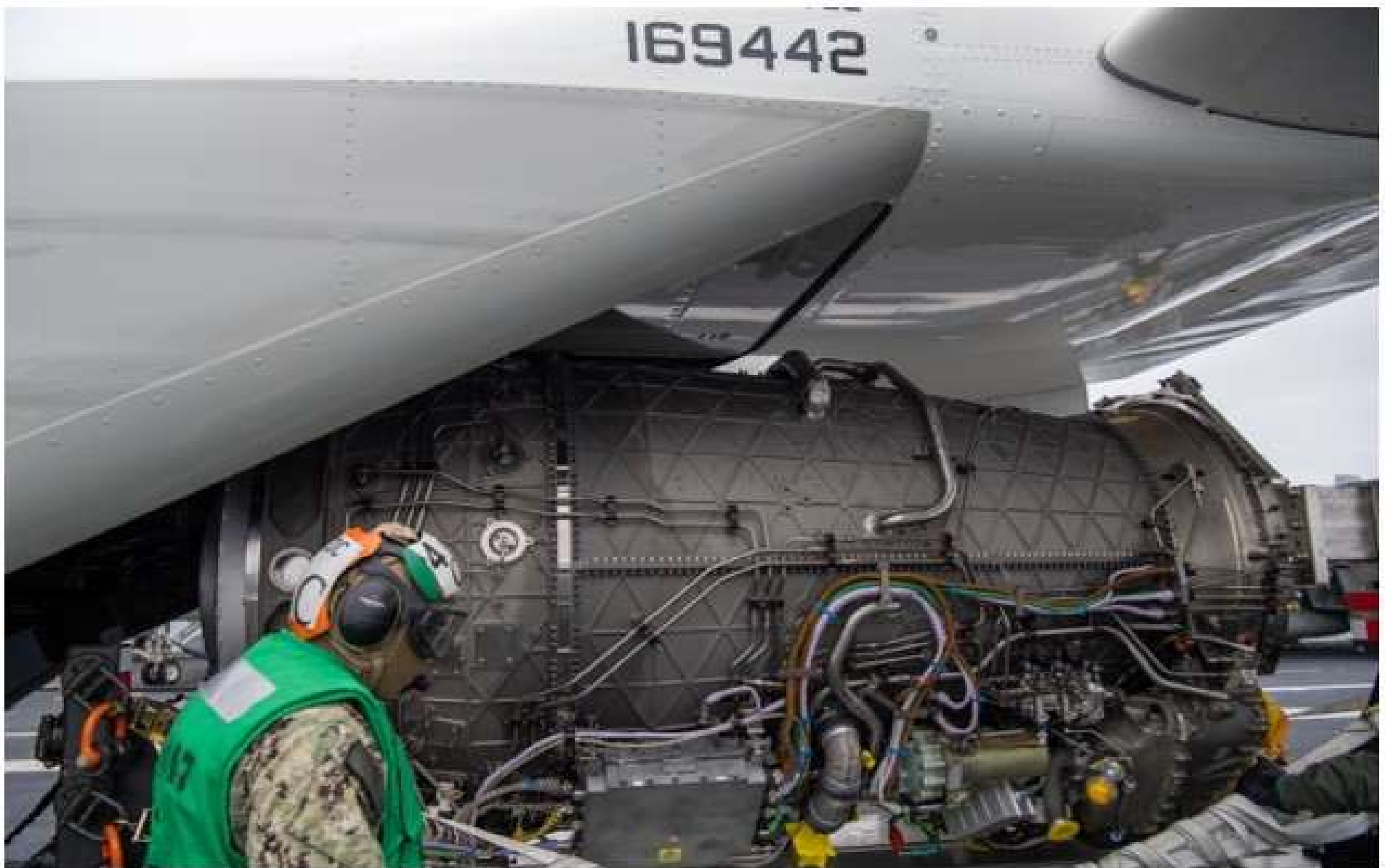
210211-N-MD461-1094 PACIFIC OCEAN (Feb. 11, 2021) Sailors assigned to the "Argonauts" of Strike Fighter Squadron (VFA) 147 load an F-35C Lightning II power module onto a CMV-22B Osprey assigned to the "Titans" of Fleet Logistics Multi-Mission Squadron (VRM) 30 on the flight deck of Nimitz-class nuclear aircraft carrier USS Carl Vinson (CVN 70). Vinson is currently underway conducting routine maritime operations. (U.S. Navy photo by Mass Communication Specialist Seaman Jeffrey Kempton/Released)
