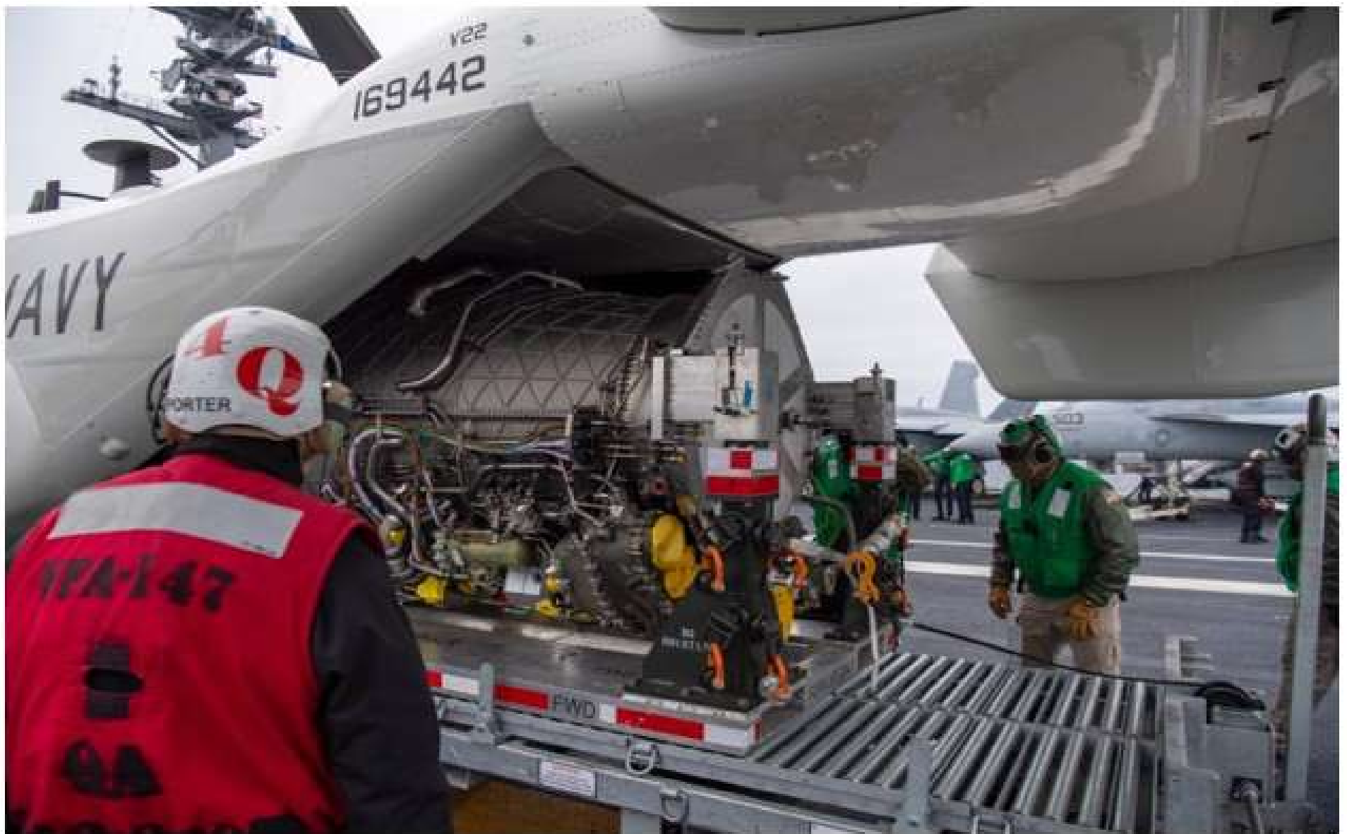
210211-N-MD461-1164 PACIFIC OCEAN (Feb. 11, 2021) Sailors assigned to the "Argonauts" of Strike Fighter Squadron (VFA) 147 load an F-35C Lightning II power module onto a CMV-22B Osprey assigned to the "Titans" of Fleet Logistics Multi-Mission Squadron (VRM) 30 on the flight deck of Nimitz-class nuclear aircraft carrier USS Carl Vinson (CVN 70). Vinson is currently underway conducting routine maritime operations. (U.S. Navy photo by Mass Communication Specialist Seaman Jeffrey Kempton/Released)
