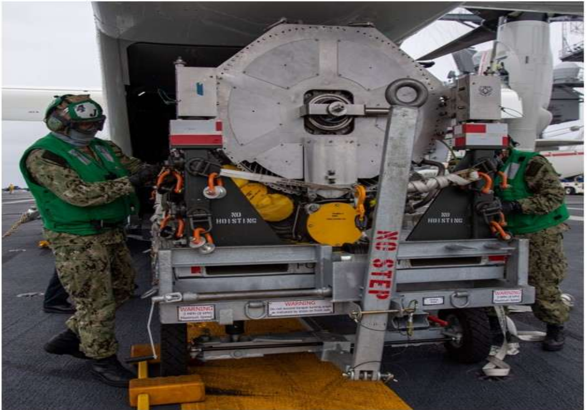
210211-N-MD461-1125 PACIFIC OCEAN (Feb. 11, 2021) Sailors assigned to the "Argonauts" of Strike Fighter Squadron (VFA) 147 load an F-35C Lightning II power module onto a CMV-22B Osprey assigned to the "Titans" of Fleet Logistics Multi-Mission Squadron (VRM) 30 on the flight deck of Nimitz-class nuclear aircraft carrier USS Carl Vinson (CVN 70). Vinson is currently underway conducting routine maritime operations. (U.S. Navy photo by Mass Communication Specialist Seaman Jeffrey Kempton/Released)
